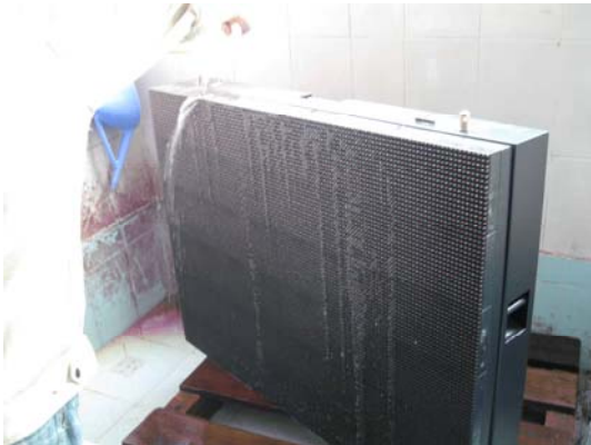
Jet Water Test
