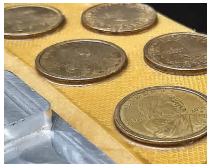
The mesh product captures additional wax material in the web and aides in holding irregular shape parts. Typically additional holding force can be attained with this material.
