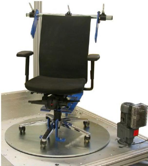
Rotation test rig for caster testing
