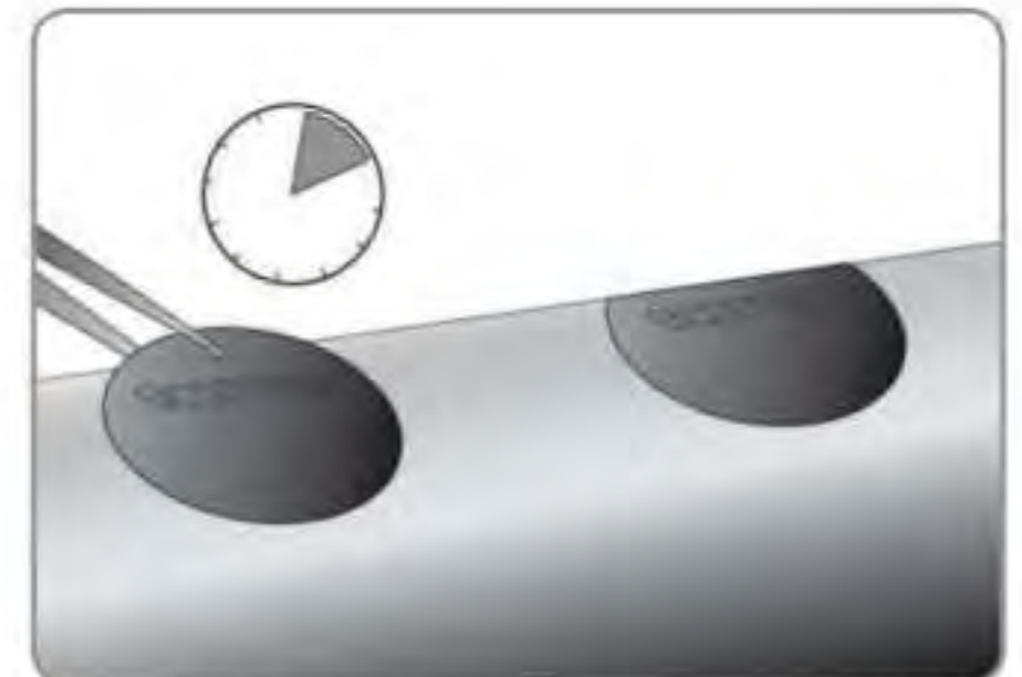
6. As each filter paper remains on the surface for two minutes, multiple tests can be undertaken at the same time, reducing inspection times further.
