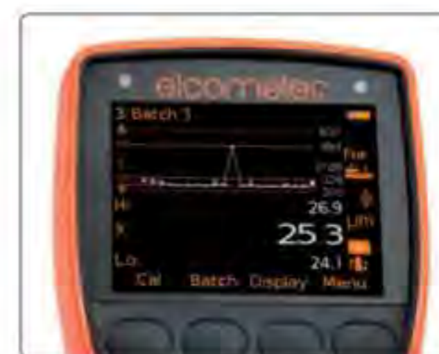
The Run Chart displays the average thickness as well as the highest and lowest readings for each scan
