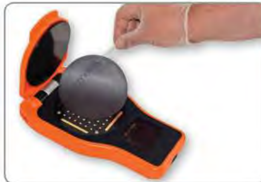
5. After two minutes, carefully remove the filter paper and magnetic disc from the test surface and place on to the measurement electrodes.
