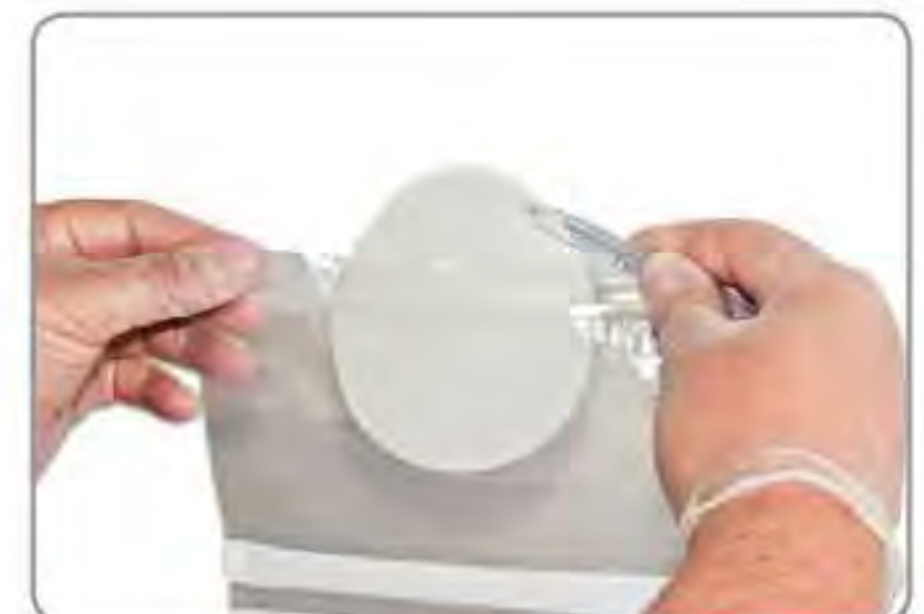
9. If required for further analysis, place the filter paper in a resealable bag (supplied).
