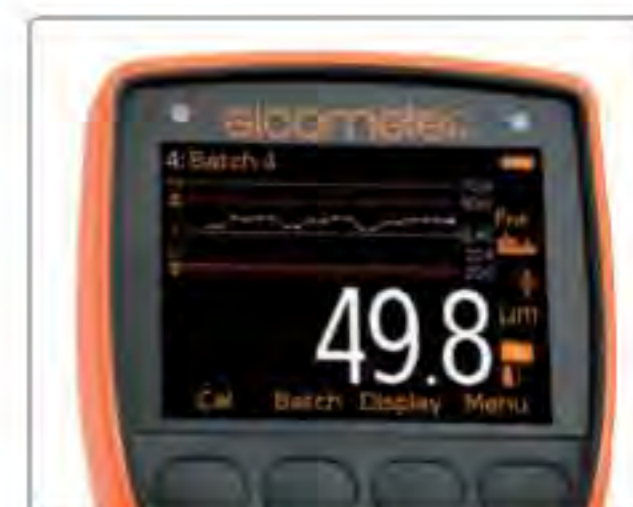
The Run Chart displays each individual reading allowing the user to identify any significant trends
