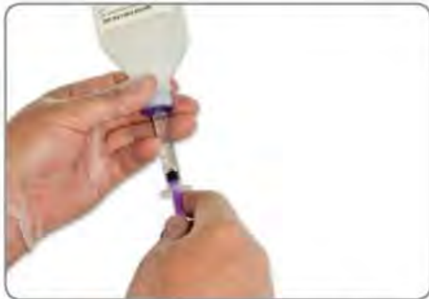
1. Wearing clean disposable gloves (supplied), fill a syringe with precisely 1.6ml of deionised water.
