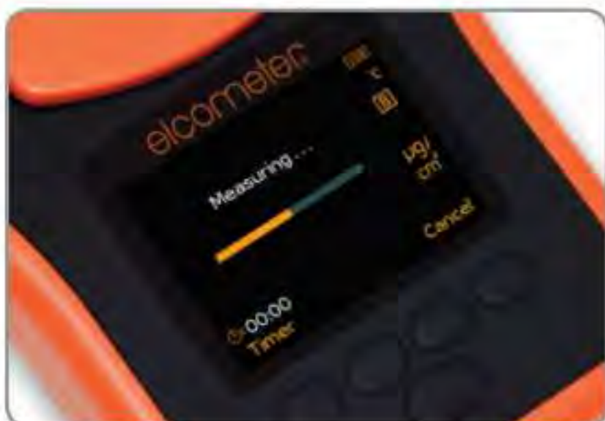
7. Close the lid, ensuring that the magnetic catch is fully engaged, the gauge will begin measuring.
