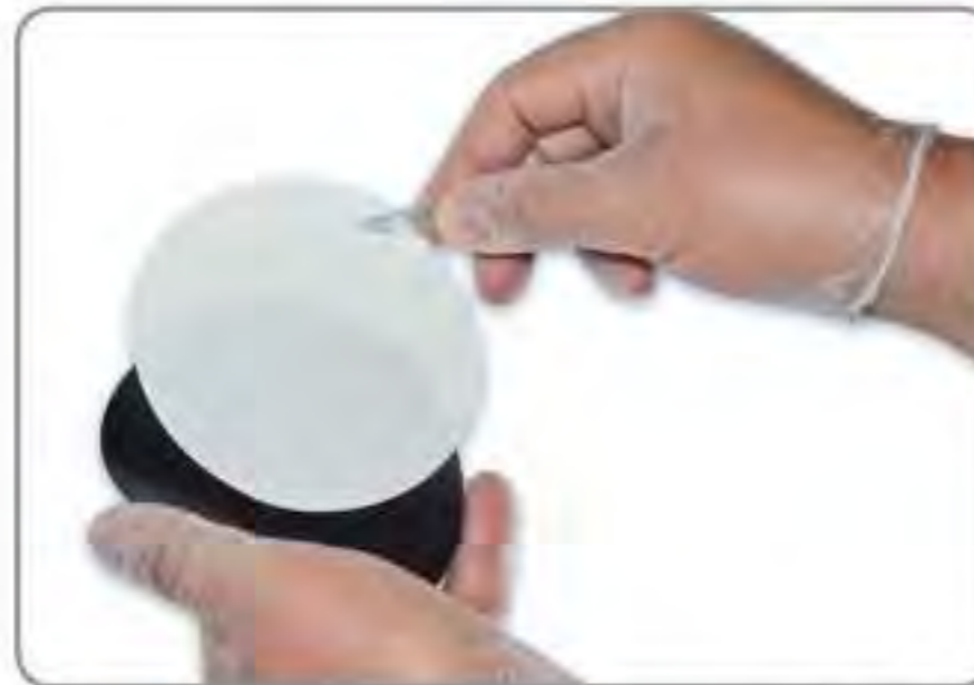
2. Using tweezers, remove a filter paper from the pack and place it on the cleaned, non-labelled side of the magnetic disc supplied.
