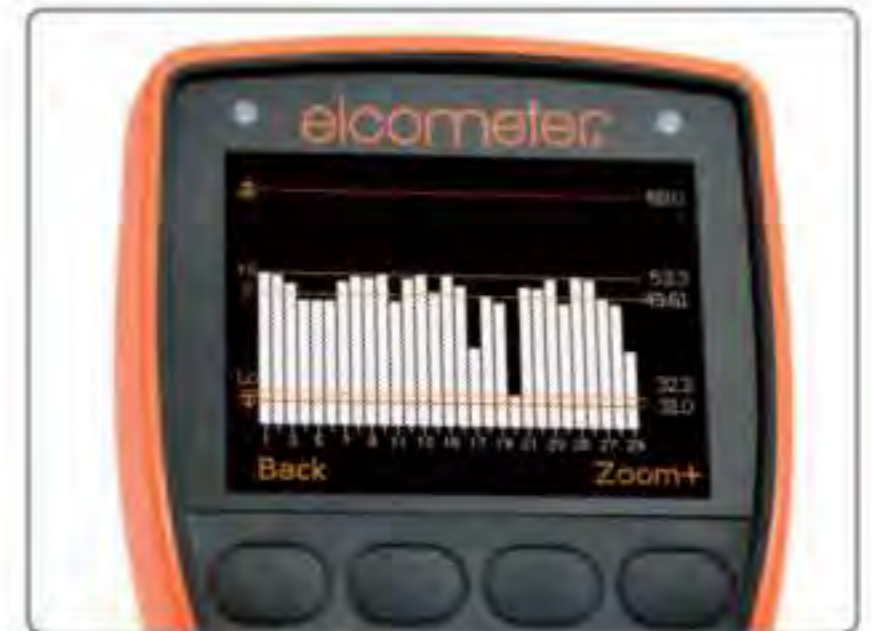
Individual batch readings can be reviewed numerically or graphically
