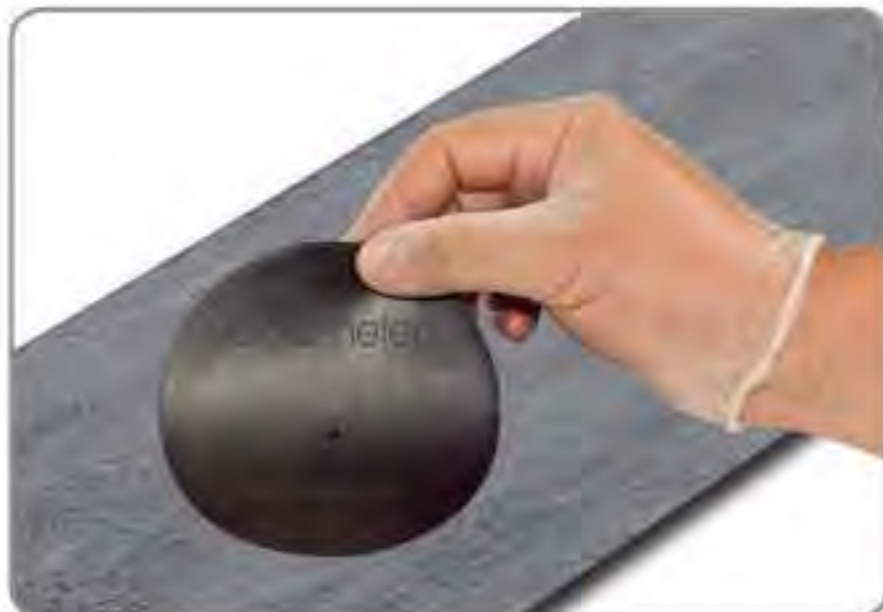
4. Place the magnetic disc, with wetted paper face down on to the area under test, pressing firmly into any contours or irregularities and start the 2 minute timer on the gauge.
