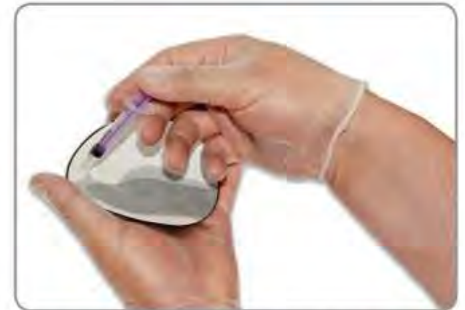
3. Disperse the water from the syringe, evenly across the whole of the filter paper and remove any bubbles from under the paper.
