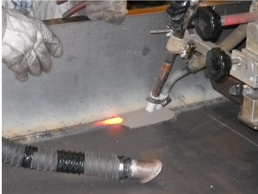
Automated submerged arc welding
