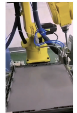
Gluing of control cabinet doors
