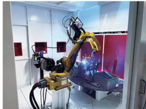
Welding of New Energy Electric Bicycle Frame
