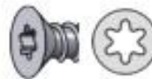
Torx A six-pointed star pattern, specifically designed to prevent cam-out and stripped heads.
