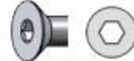
Socket, Hex or Allen A hexagonal hole for use with an Allen wrench.
