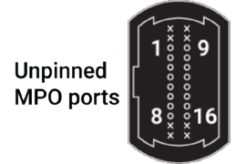
Figure 11: MPO-24 port configuration with 16 fibers
