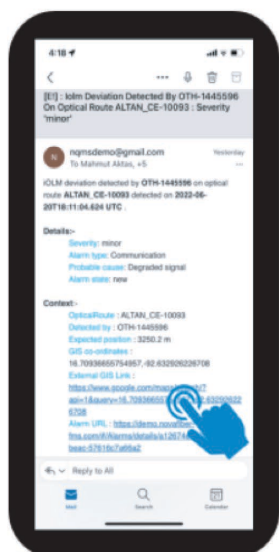
Email notification with a Google Maps™ links to the point of failure
