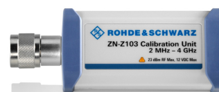
One-step calibration with automatic calibration unit (R&S®ZN-Z103)
