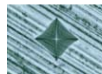
Indentation on an abrasive material
