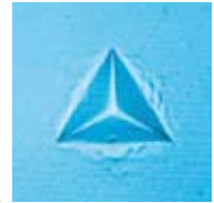
Indentation by triangular pyramid indenter
