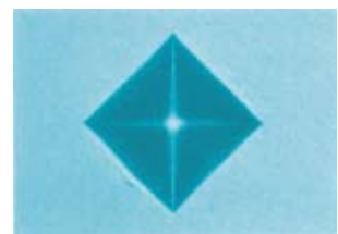
*Surface indentation on a structural material
