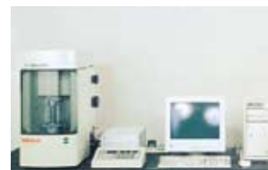
Rockwell hardness standard testing machine SHT-31 (Special accessories except the main unit and operation panel)
