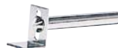
19BAA202 Butt laying gage (Standard accessory) Can improve work efficiency when it is used for repeated measurement of the same location on workpieces of the same shape and size. You can locate a workpiece at the correct location just by lightly locating the work against the stop attached to the frame.
