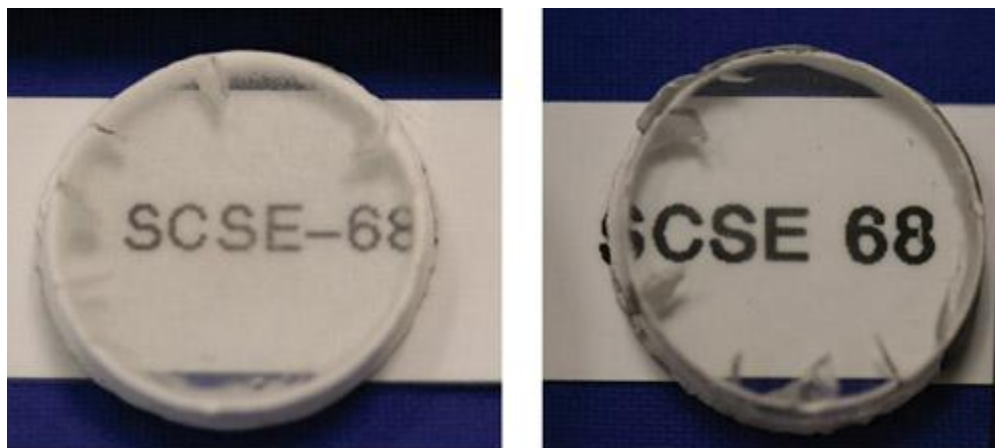
Production of 15-millimeter-diameter samples of transparent ceramic yttrium– aluminum–garnet. A sample exhibits excellent optical qualities after hot isostatic pressing (right).
