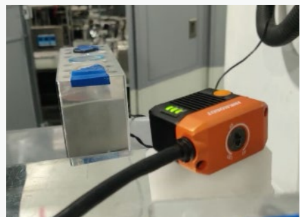
Lithium battery color detection
