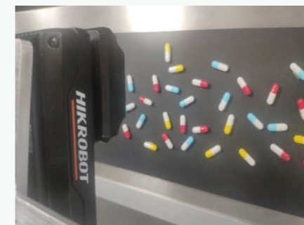
Dynamic tracking and counting during pill packaging
