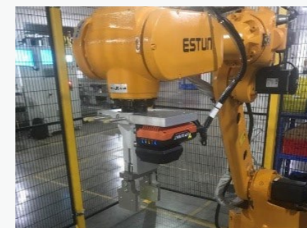
Robotic arm guided product gripping
